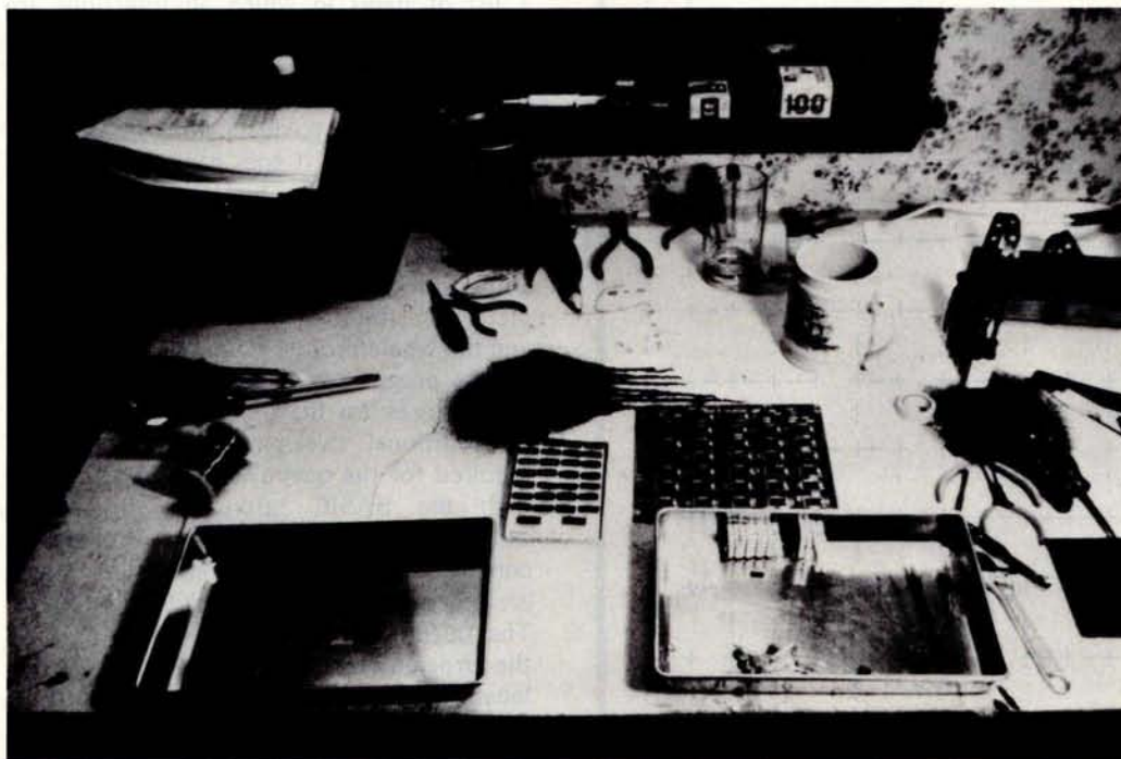
Photo 7b: As the parts are checked off against the parts list, they are moved from the pan at the left into the pan at the right, and arranged in order for access later during assembly. In this photo, the circuit board for the new module and a conductive foam pad with the integrated circuit parts are both placed at the back of the two pans.
