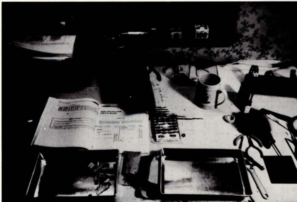
Photo 7a: A good practice when assembling complicated kits is built into the Heathkit manuals: a parts check off. In this photograph, the parts for the "RAM and counter circuit board" have been unpacked from the paper bags, with loose parts placed in the baking pan at the left.
