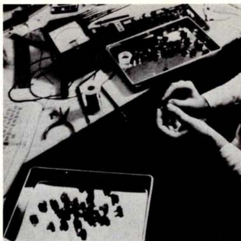
Photo 3: One of the most tedious tasks when assembling the H9 is manually checking each switch of the keyboard. Here, two metal cake pans are used as input (background) and output (foreground) of the process of checking each switch with an ohmmeter.
